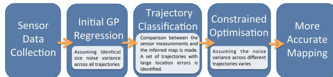
Figure 2: Our algorithm applies GP regression and constrained optimisation to achieve an accurate mapping of the environment parameters of interest.
