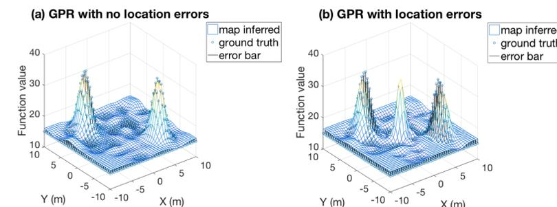
Figure 4: (a) shows the map generated by GP regression if all trajectories are accurate. This can be considered as the best mapping result we can achieve. (b) illustrates a fake peak (middle) is generated by applying standard GP regression directly to the sensor data with inaccurate location information.
