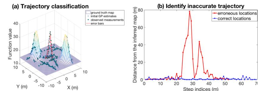
Figure 5: (a) Differences between the observed function values and the inferred map from the initial GP regression is computed. (b) Trajectories with high values of difference are classified as inaccurate.
