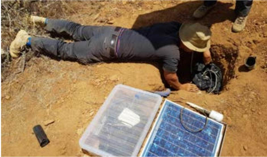
We used seismometers buried in the ground to detect the vibrations made by elephants. This image shows us installing a seismometer.
